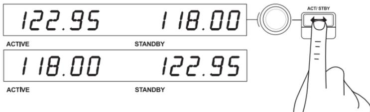
To adjust the radio stack frequencies, first select the radio mode using the radio mode selector knob on the left of the panel. Using the rotary controls to the right of the LED screen, adjust the values of the standby frequency on the right side of the screen. The outer rotary adjusts standby frequency by increments of 1 and the inner rotary adjusts decimals. Please note, you can only adjust the standby values and not the active values.
